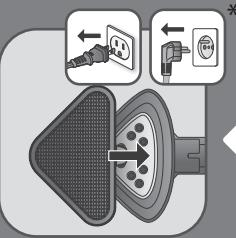
**EN** The steam bonnet mesh filters the water impurities and protects textiles from water drops.
