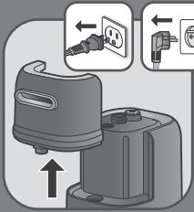
**EN** Unplug, then remove the water tank.
