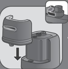
**EN** Screw back the cap and place the water tank back to its appliance.
