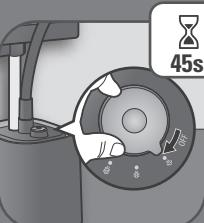
**EN** Turn the On/Off Button, in order to switch on the appliance. Then, adjust steam output by turning the button.
