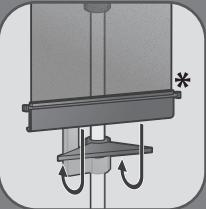
**EN** Unwind the support and fix it, by adjusting the tension with the dedicated hook and lock it.
